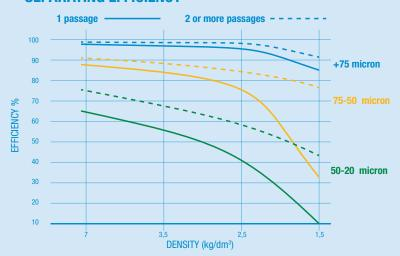
The given indications of separation efficiencies are a combined result of theoretical calculations and in field experience. Expected separation efficiency may also depend on the shape of actual particles, pressure loss and other factors.
